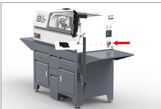
Figure 5-23: The Main Disconnect switch on the side of the machine's electrical cabinet.
