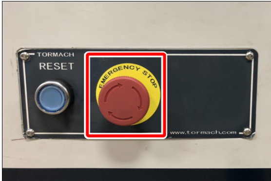
Figure 5-25: Emergency Stop button.
