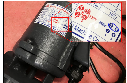
Figure 5-40: Coolant pump motor jumper configuration diagram.
