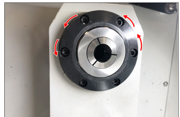
Figure 5-35: Spindle rotating counterclockwise, in the correct forward direction.
