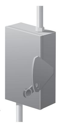
The wire gauge used from the breaker box to the outlet must be of sufficient size to handle the amperage of the kiln for a given distance. We recommend a wire gauge to be used that is good for up to 50 ft. As electricity flows over distances it can lose voltage in the form of heat. If the gauge of the wire is increased the amount of loss decreases. This is why we recommend increasing the recommended wire gauge for every 50 ft. of run.
