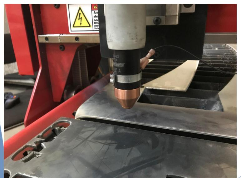
Touches the material, using grounding to sense initial height (ohmic sensing)
