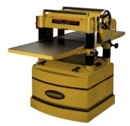
The Planer is used to flatten the surface of a board and its adjacent edge.
